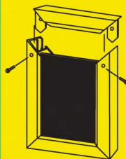
2 front mounted security screws. Benefits: Easy and fast removal of screws with hand or cordless tools. Great for frequent insert changes
